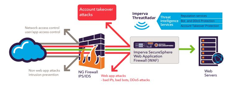
Figure 2: Imperva SecureSphere Web Application Firewall with ThreatRadar
